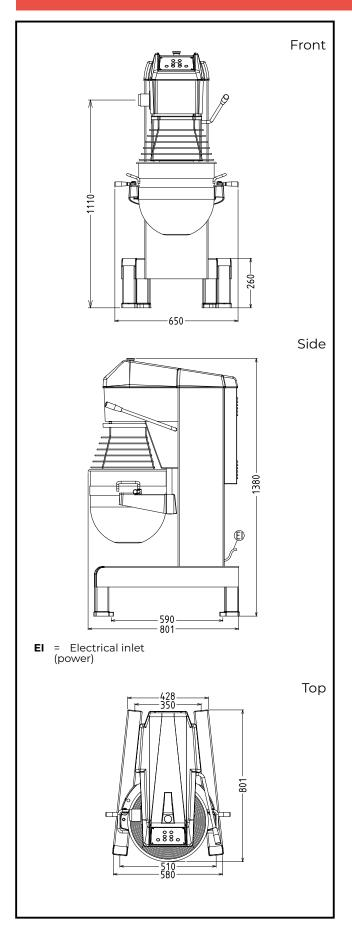
Electric Supply voltage: 200-240 V/1N ph/50/60 Hz **Electrical power max.:** 2.2 kW **Total Watts:** 2.2 kW Capacity: Performance (up to): 10 kg/Cycle **Capacity:** 40 litres Key Information: External dimensions, Width: 655 mm External dimensions, 850 mm Depth: External dimensions, Height: 1370 mm **Cold water paste:** 10 kg with Spiral hook 70 with Whisk Egg whites:
